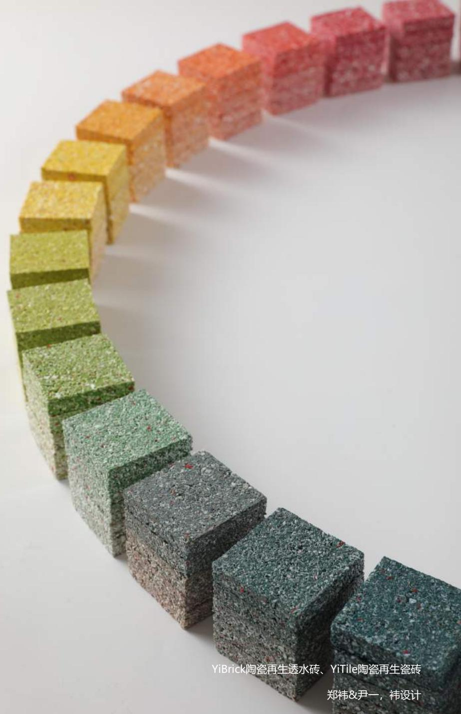
YiBrick陶瓷再生透水砖、YiTile陶瓷再生瓷砖
